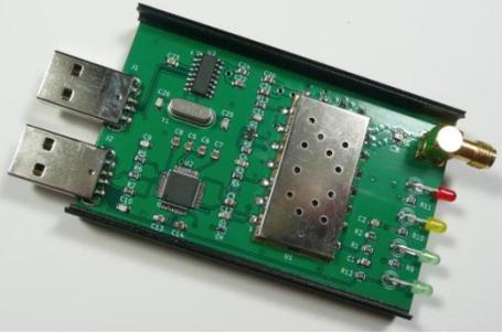
A green printed circuit board (PCB) with various components, including two USB connectors on the left and a SMA connector on the right, is shown being inserted into a black extrusion case half. |
