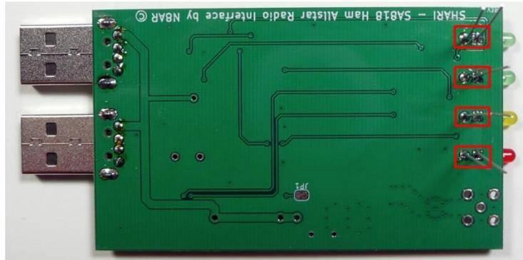
Trim the excess lead length of all 4 LEDs
