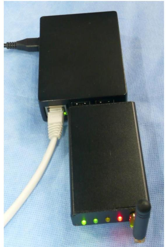
Figure 1 - SHARI Plugged Into a Raspberry Pi
