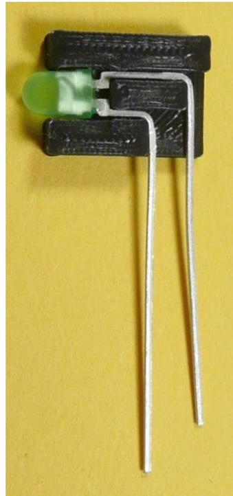
Both leads bent and ready for installation
