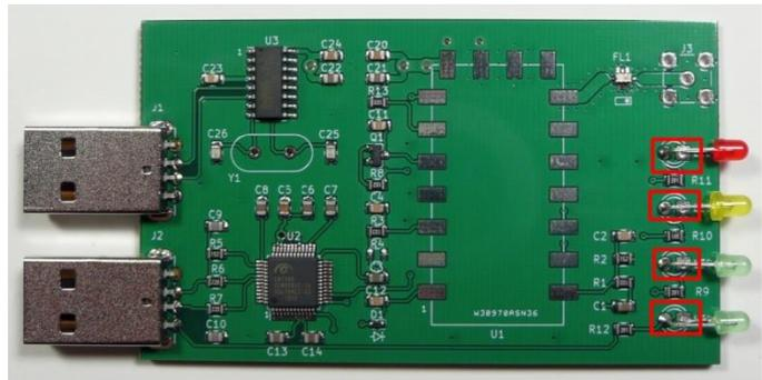
Insert the crystal, Y1, into the PC board from the top as shown in the photo. Solder the two pins on the bottom side of the board. Trim excess lead length.
