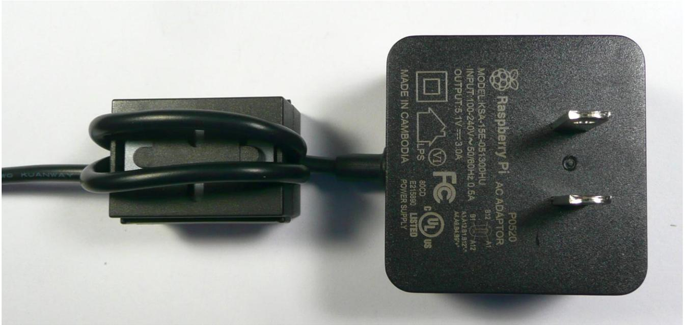
**Split Core Ferrite Installed on Raspberry Pi Power Supply Cable (three turns)**
