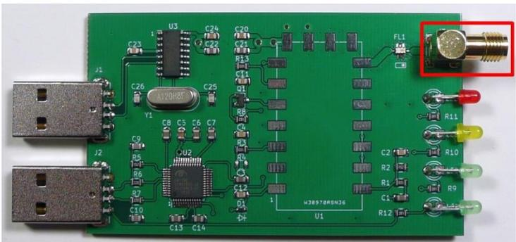
Next, you will solder the SA818 radio module to the PC board in the U1 position. You will solder 18 castellated holes on the module edges to the pads on the PCB. If you have never soldered castellated holes before, please go to
