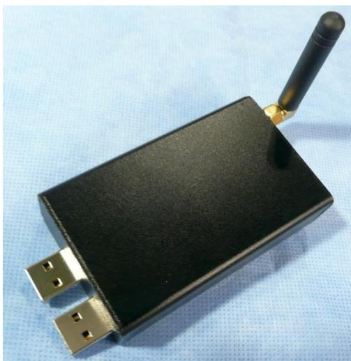
Figure 2 – SHARI has Two Type A Male USB Connectors for the Allstar Interface and Radio Programming
