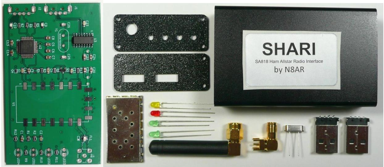
Figure 5 – SHARI Kit Components (included ferrite filter not shown)
