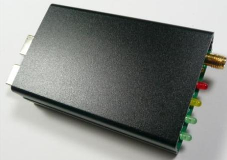
The final assembled SHARI device, showing the black extrusion case fully closed around the green PCB, with the USB connectors and SMA connector visible.                                          |
