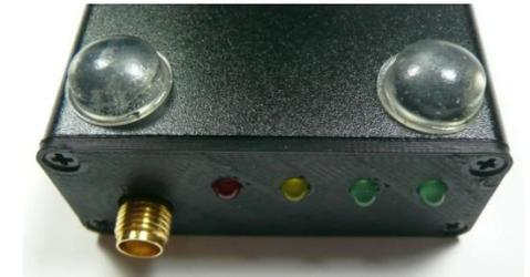
Apply the "SHARI" label and attach the antenna to the SMA connector.
