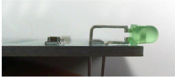
While holding the LEDs so they do not fall out, turn the board over on a flat surface. Align the LEDs so they are perpendicular to the end of the board. Ensure that they protrude an equal length from the board and that the annular rings at the base of the LEDs do not protrude beyond the edge of the board.
