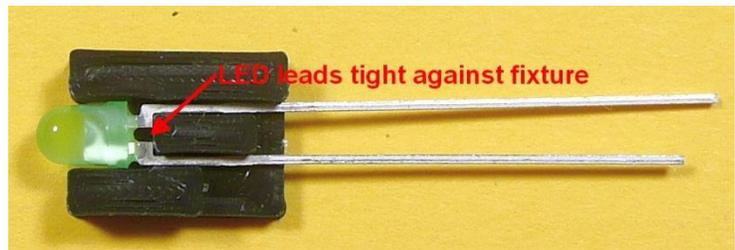
Grasp the short lead and bend it 90 degrees as shown in the photo. Be sure it bends tight against the fixture
