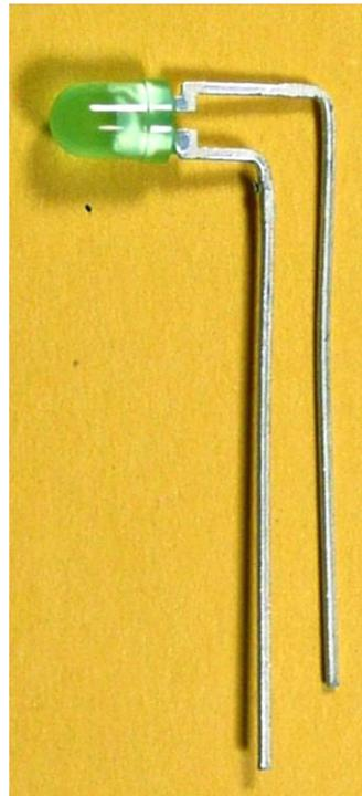
Insert the first green LED with the newly formed leads into the LED4 position on the board and position it as shown in the photo to the right. Note that the largest diameter part of the LED body is touching the PC board. Repeat for LED1 (green), LED2 (yellow) and LED3 (red)
