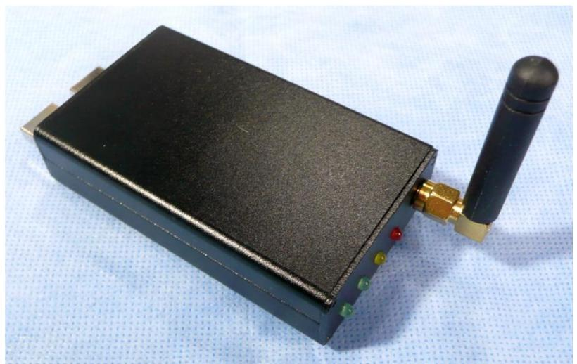
Figure3 – Four LEDs indicate the Status of Power, Allstar USB Interface, Radio COS and Radio PTT
